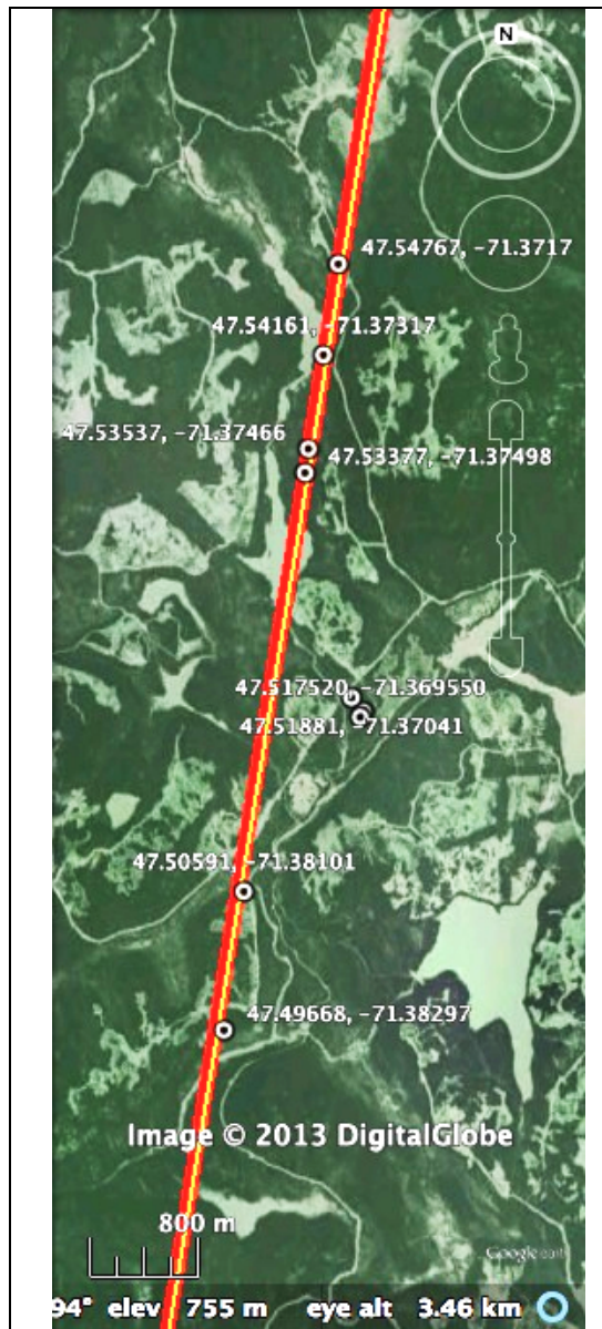
Enlargement of 2011 Eco3D SIMPL flight line 1 (yellow), flight path (red) and field plots (circles) on Sept. 1, 2011 in southeast Quebec.
